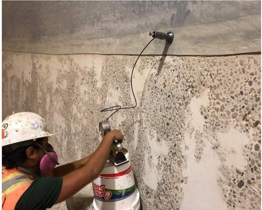
Quality Assurance testing – adhesion strength pull-off testing.
