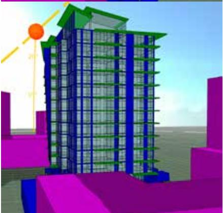
The images are examples of the graphical output from modelling software (IES VE - <https://www.iesve.com/>), and convey the relationship of buildings to surrounding structures while taking into account solar effects on the building form and façade.
