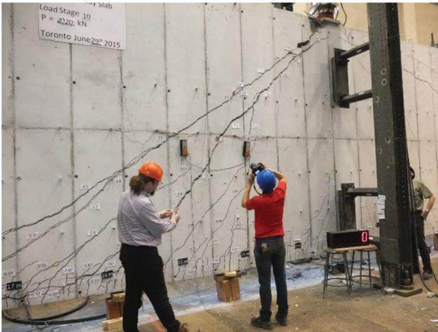
(b) Failure at  $P = 2162 \text{ kN}$  (486 kips)
