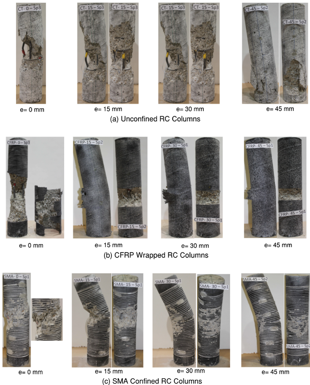
Fig. 6. Failure modes of unconfined, CFRP-wrapped, and SMA-confined RC columns tested at e = 0 mm, e = 15 mm, e = 30 mm, and e = 45 mm.
