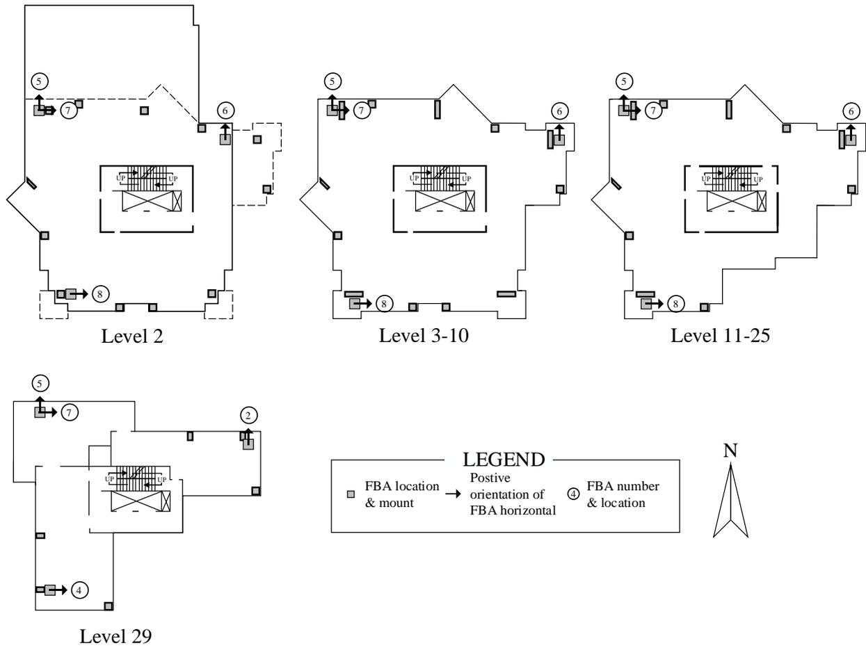
Figure 4: Sensors layout at different levels
