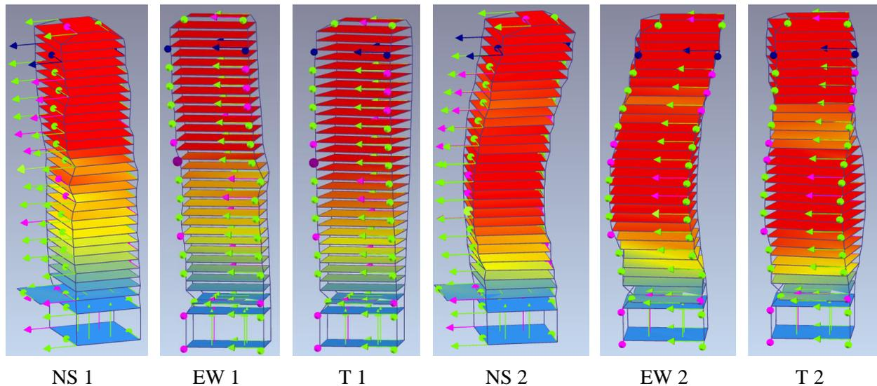
Figure 6: The first six mode shapes from the ambient vibration test.
