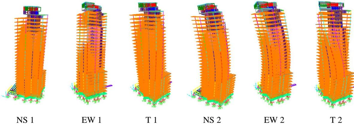
Figure 8: The first six mode shapes from the FE model without the basement
