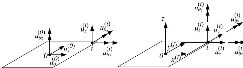
Figure 1: Master-slave diaphragm assumption. Left: 6 degrees of freedom node. Right: slave node with 3 degrees of freedom.
