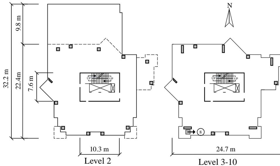
Figure 3: Level 2 (left) and level 3-10 (right) floor layout of the City Crest Tower.
