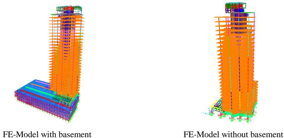
Figure 7: The two FE-models with and without the basement.
