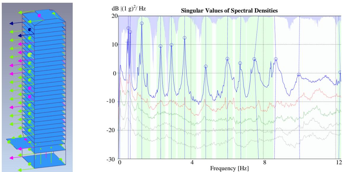
Figure 5: Computer model in ARTEMIS for the Operational Modal Analysis (left) and the singular values of spectral densities (right).
